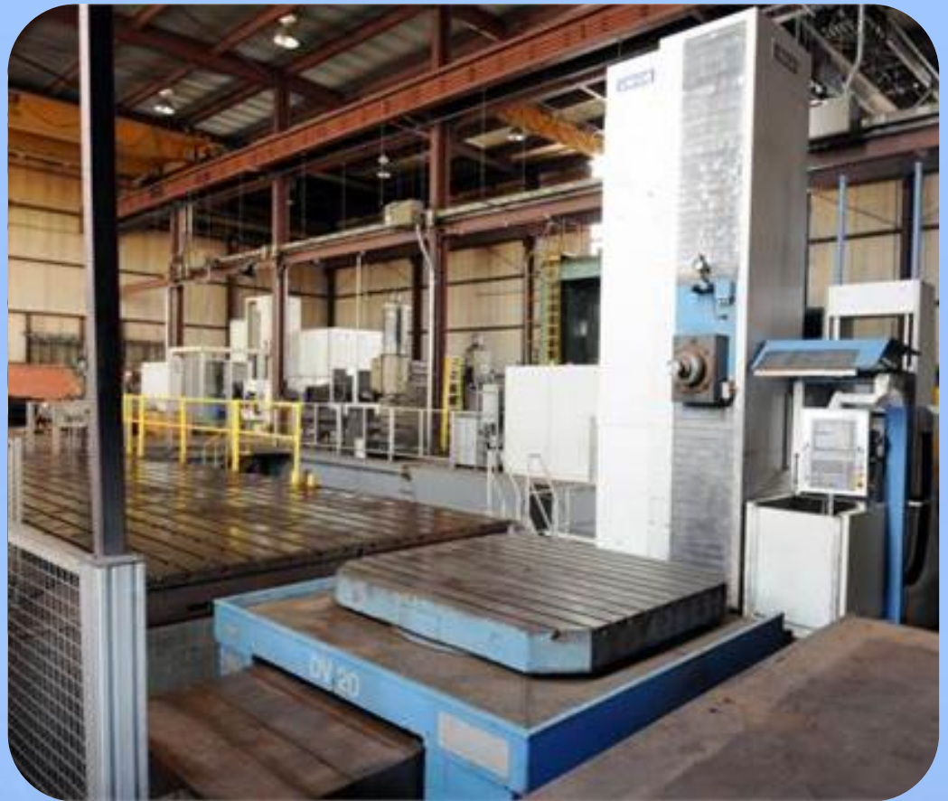
Union P150 Horizontal Mill with a Rotary Table and 7 Axis Heidenhain Control for Extreme Versatility
